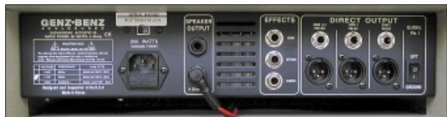
Three direct outs grace the Shenandoah’s back panel.
